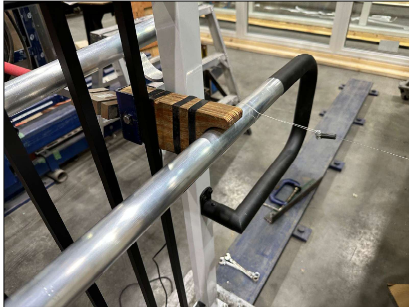
Figure 1 – Horizontal Concentrated Load on Mounting Bracket
