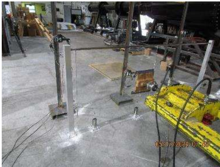
Photo No. 1 In-Fill Load Test at Center Edge of Glass Panel
