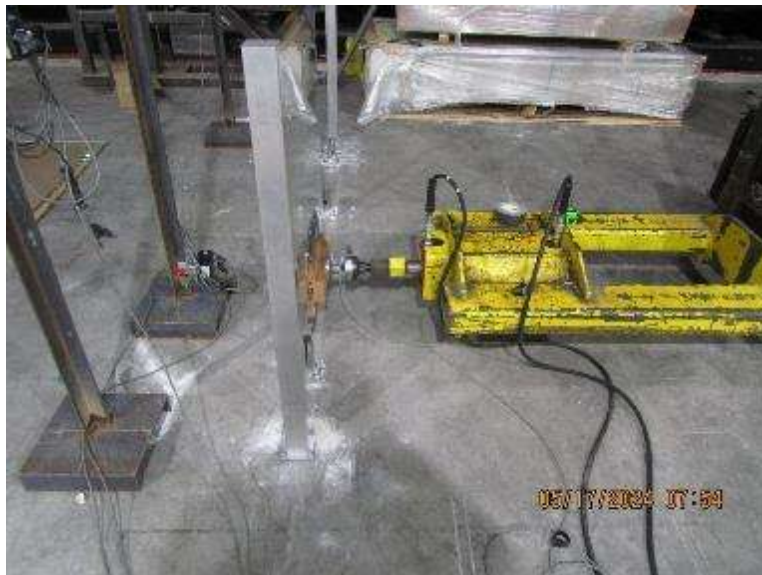
Photo No. 2 In-Fill Load Test at Bottom of Glass Panel
