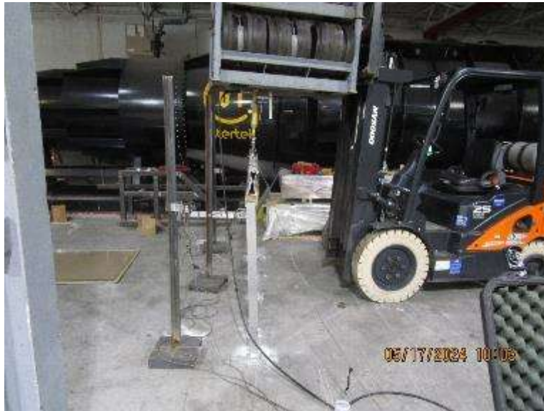
Photo No. 5 Vertical Uniform Load Test on Top Rail
