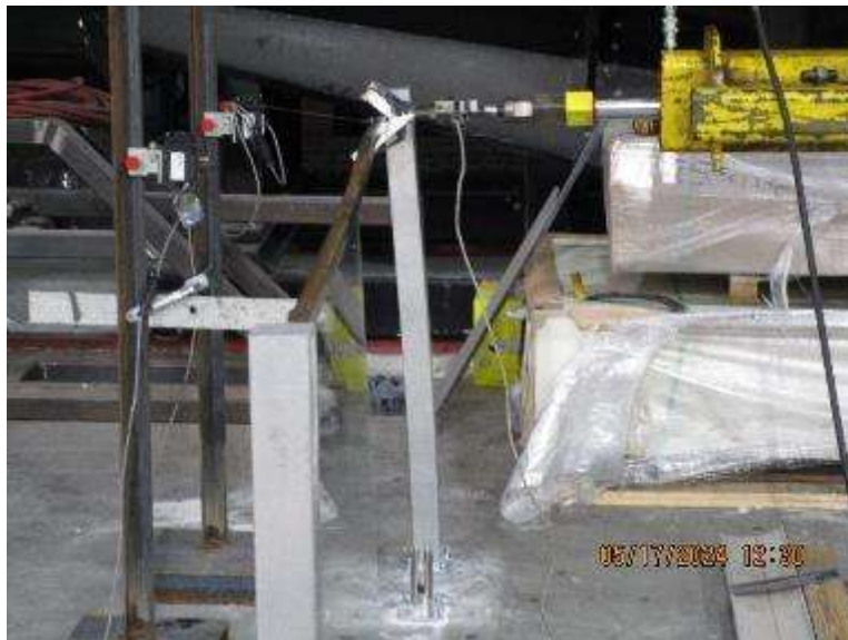
Photo No. 6 Concentrated Load Test at Top of Post
