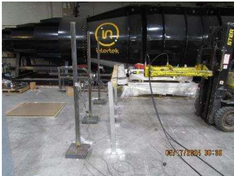
Photo No. 4 Horizontal Uniform Load Test on Top Rail
