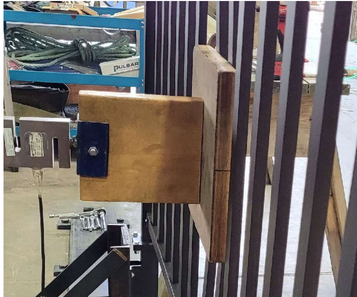
Figure 1. In-fill Load Test
