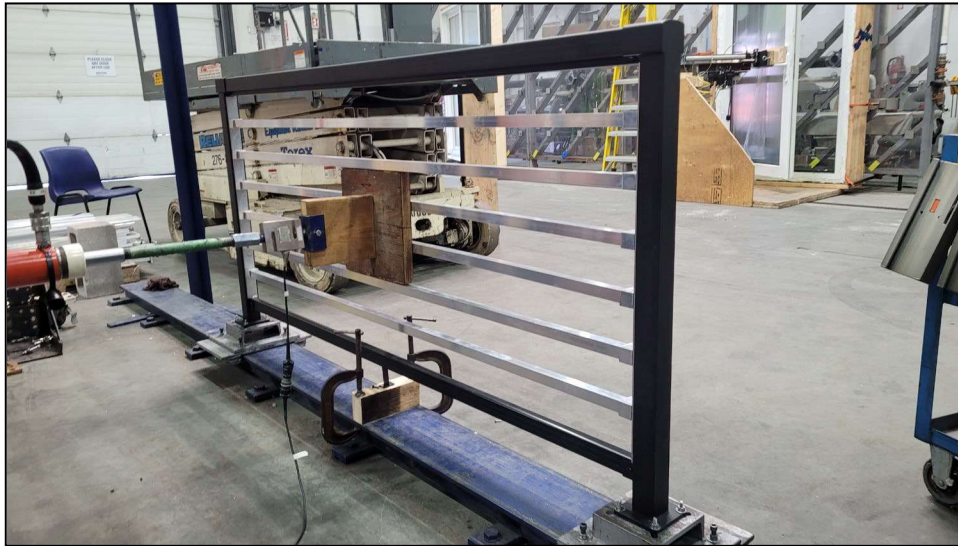
Figure 1. In-Fill Load Test
