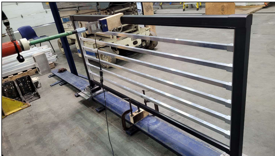
Figure 2. Midspan of Top Rail Concentrated Load Test
