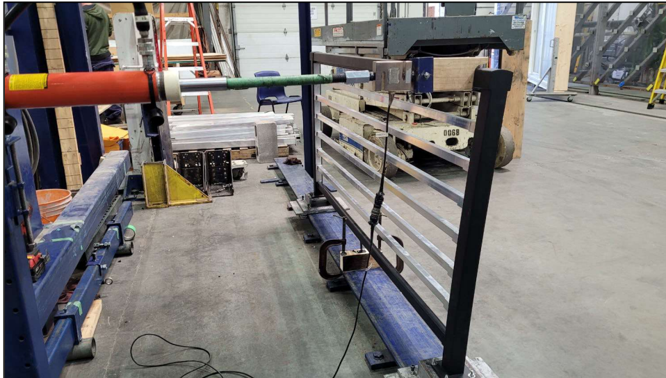
Figure 3. Adjacent to Post Connection Concentrated Load Test
