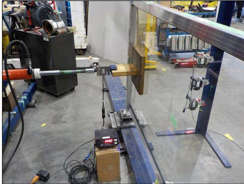
Figure 1. In-Fill Load Test
