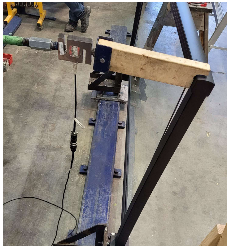
Figure 4. Horizontal – Top of Post Concentrated Load
