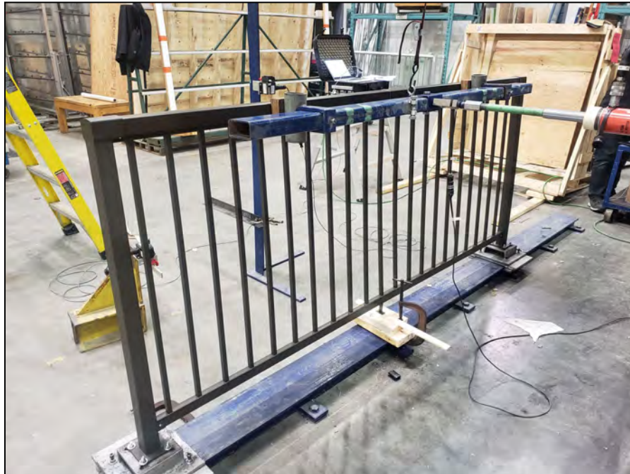
Figure 3 – Horizontal Uniform Load Test
