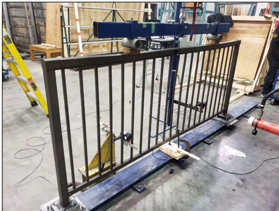
Figure 2 – Vertical Uniform Load Test
