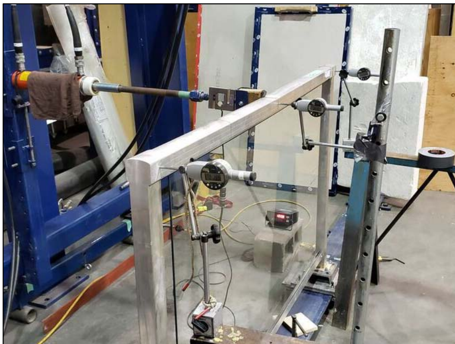
Figure 10. 5 ft. Vista Aluminum Glass Railing System Horizontal – Mid-Span of Top Rail Concentrated Load
