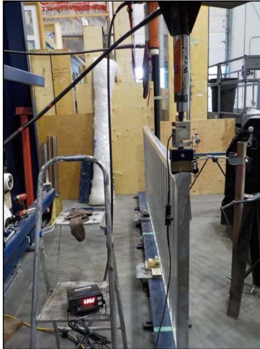
Figure 5. 8 ft. Vista Aluminum Wide Picket Railing System Vertical – Top Of Post Concentrated Load
