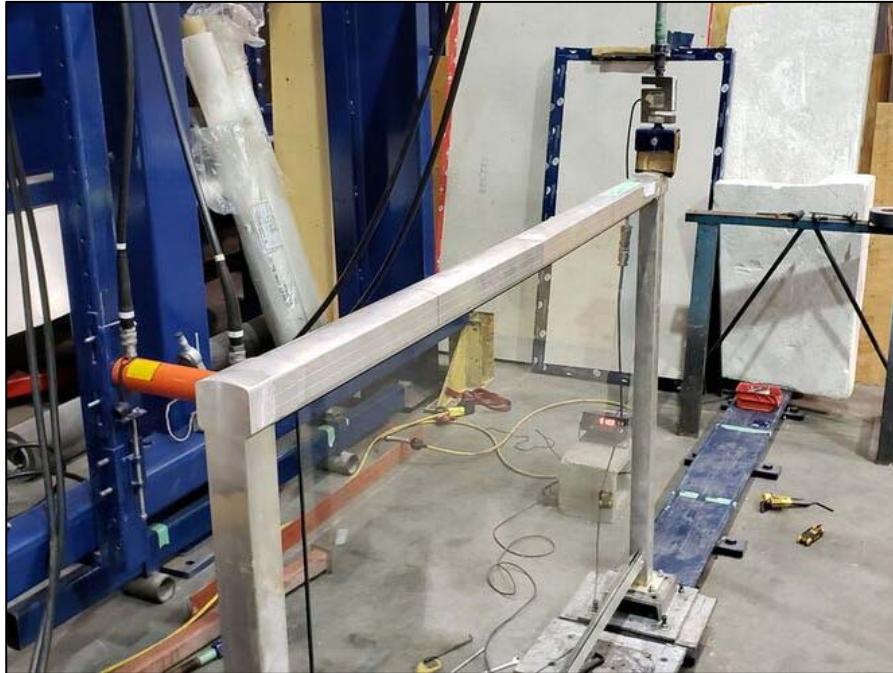
Figure 9. 5 ft. Vista Aluminum Glass Railing System Vertical – Top of Post Concentrated Load
