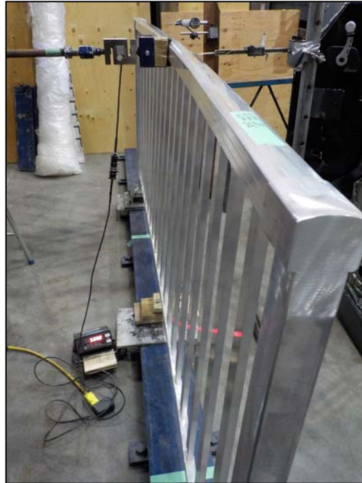
Figure 7. 8 ft. Vista Aluminum Wide Picket Railing System Horizontal – Mid-Span of Top Rail Concentrated Load
