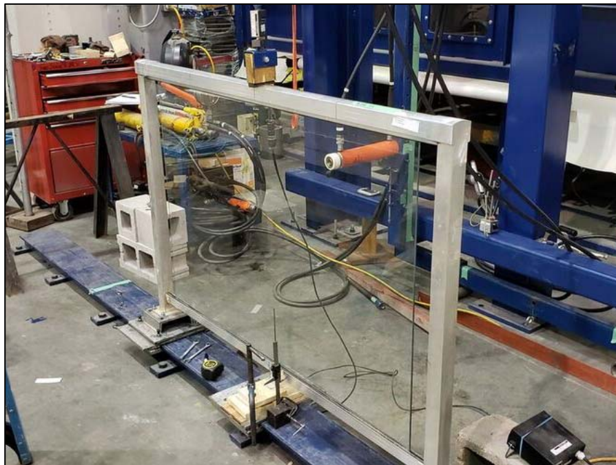
Figure 8. 5 ft. Vista Aluminum Glass Railing System Vertical – Mid-Span of Top Rail Concentrated Load
