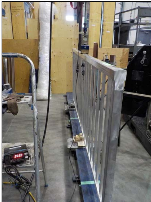
Figure 6. 8 ft. Vista Aluminum Wide Picket Railing System Vertical – Mid-Span of Top Rail Concentrated Load
