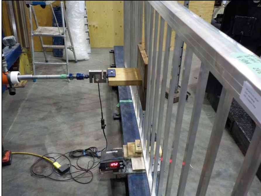
Figure 1. 8 ft. Vista Aluminum Narrow Picket Railing System – In-Fill Load Test
