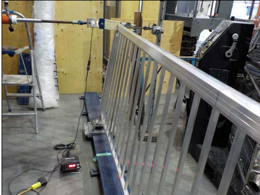
Figure 3. 8 ft. Vista Aluminum Narrow Picket Railing System Horizontal – Top Rail Adjacent to Post Connection Concentrated Load
