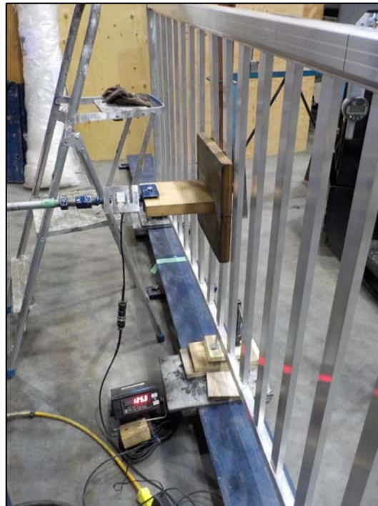
Figure 4. 8 ft. Vista Aluminum Wide Picket Railing System – In-Fill Load Test
