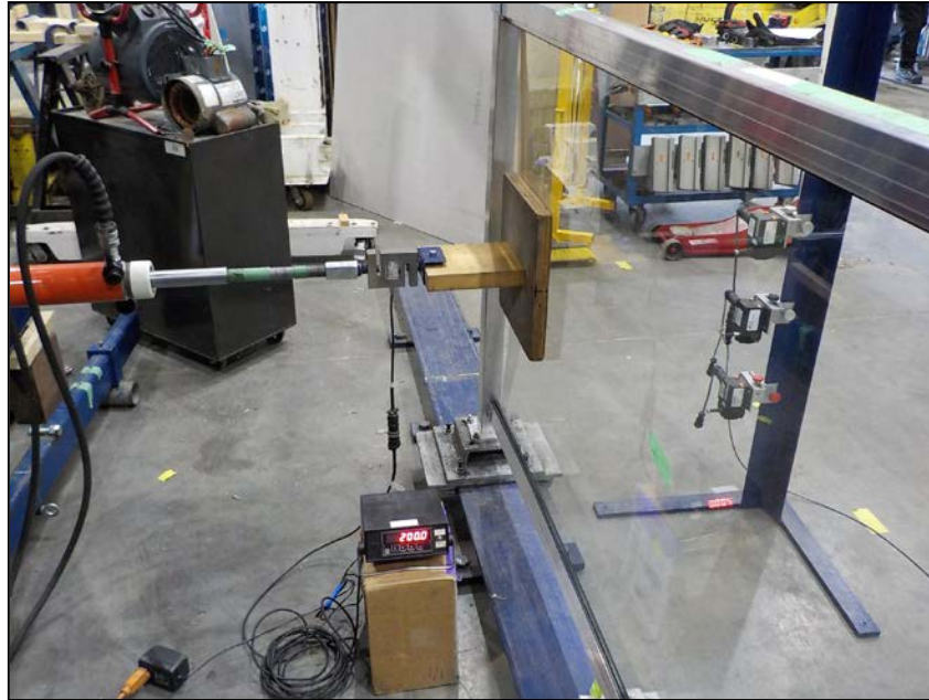
Figure 1. In-Fill Load Test
