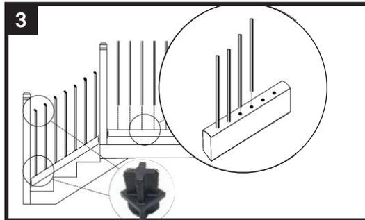
3 With a high-quality polyurethane construction adhesive, fill all the holes half way. Insert balusters into pre-drilled holes in rail. This will bond the wood to the balusters. Best to use 26" baluster option for stairs.
