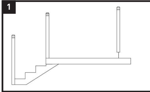
1 Set newel posts (sold separately) to accommodate pre-drilled rail length. Centre pre-drilled rail between newel posts and trim equal amounts from each end of top and bottom rails.
