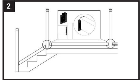
2 Slide rail hanger bracket over the end of the rail and attach with screws through end of rail. (Hint: Opening of bracket must always be up).
