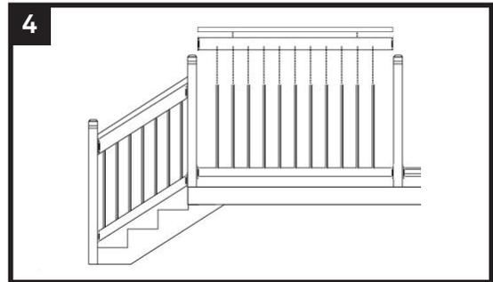
4 Apply pre-drilled top rail. Attach cap rail. Fasten railing section to post with rail hanger brackets.
