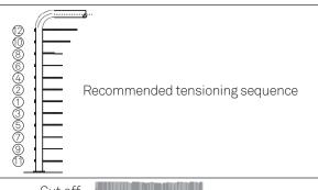
3. When all of the cables are tight, cut off any exposed thread as near to the locknut as possible by using a cut-off wheel or hack saw.
