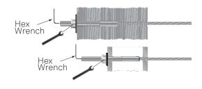
2. Tension all cables to desired amount in sequence, beginning with the center cables, moving up and down toward the top and bottom. As you tension each cable, give it a sharp pull downward mid-span to help set the wedges, then re-tension as necessary in the same sequence.
